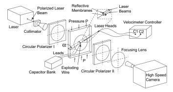
Fig. 1. Specimen configuration and experimental setup. Far-field pressure P and the inclination angle  $\alpha$  are system variables. Dynamic photoelasticity and high-speed photography were used along the optical axis. Two velocimeters measured fault-parallel particle velocity histories above and below the simulated fault. The capacitor bank and exploding wire configuration provided the rupture initiation mechanism and the synchronizing trigger.
