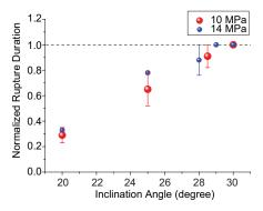
Fig. 3. Rupture duration, normalized by the maximum potential sliding time, plotted as a function of inclination angle  $\alpha$  for two values of far-field pressure P. Normalized rupture duration of 1 corresponds to crack-like ruptures, whereas smaller values correspond to progressively narrower pulse-like
