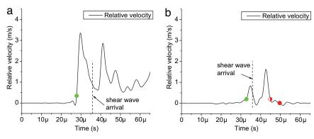
Fig. 4. Relative velocity records, at 40 mm away from the hypocenter, that capture the sub-Rayleigh to supershear transition. (a) A sub-Rayleigh crack transitioning to a supershear crack ( $\alpha = 30^{\circ}$ , P = 14 MPa). (b) A sub-Rayleigh pulse transitioning to a supershear pulse ( $\alpha = 27.5^{\circ}$ , P = 14 MPa).
